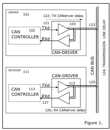
Figure 1 shows a CAN system in the process of transmitting a signal, with the CAN-frame travelling from the sender to the receiver. The CAN sender logic transmits the bit at the output TXd, indicated by 121. Signal 121 from sending CAN-controller 102 passes through CAN-driver 103 out on the CAN-bus on drop line 123, then along the CANbus to drop line 125 and to receiving CAN-driver 113, over signal line 127 to the receiving CAN-controller. This path results in a signal delay between 121 to 127.
